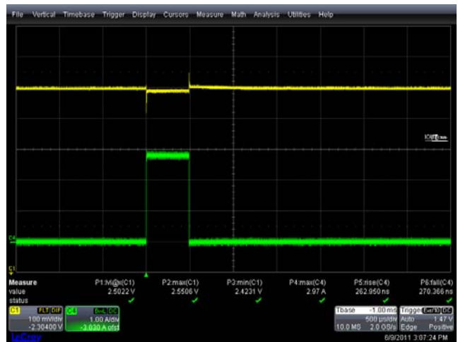
FIGURE 20. TRANSIENT LOAD RESPONSE, V_{IN} = 3.3\text{V} , V_{OUT} = 2.5\text{V} , C_{OUT} = 220\mu\text{F} , 25\text{m}\Omega
